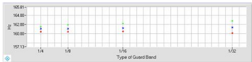
Figure 2.4 Measurement of average frequency error vs guard period at specific power level.
