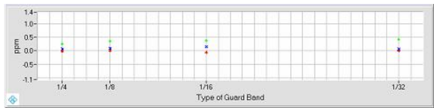
Figure 2.5 Measurement of average symbol clock error vs guard period at specific power level.
