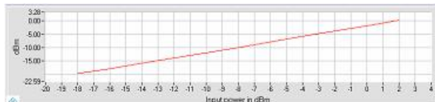
Figure 2.2 Measurement of average RMS output burst power vs input power at specific frequency.
